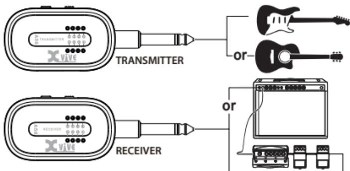
2. Pair the transmitter and receiver by making sure that they are set to the same wireless channel. A58 has six channels; use the channel select button to change the channel as needed.
