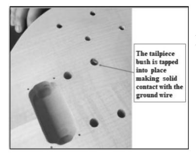
Installing the tailpiece bushing may be done with a plastic headed mallet or place a small piece of wood on top of the bushing to prevent damage and top the bushing in place with an ordinary hammer. Now screw the tailpiece mounting screws back into the bushings.
