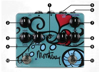
EFFECT TYPE: FUZZ, WAH, HARMONIC WAH, VIBRATO, ROTARY, OCTAVE POWER REQUIREMENT: 9VDC CENTER NEGATIVE, 75mA+ POWER SUPPLY REQUIRED INPUT/OUTPUT: MONO INSTRUMENT INPUT, MONO INSTRUMENT OUTPUT
